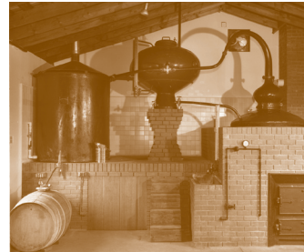
Antique cognac still. All the controls are operated by hand. It takes 48 hours to distill one barrel.
